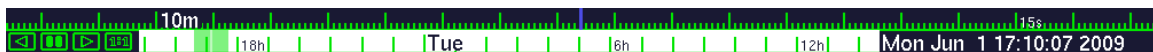
Fig 1: The GeoZui4D time bar. The top section animates as time passes. The lower section gives an overview.
